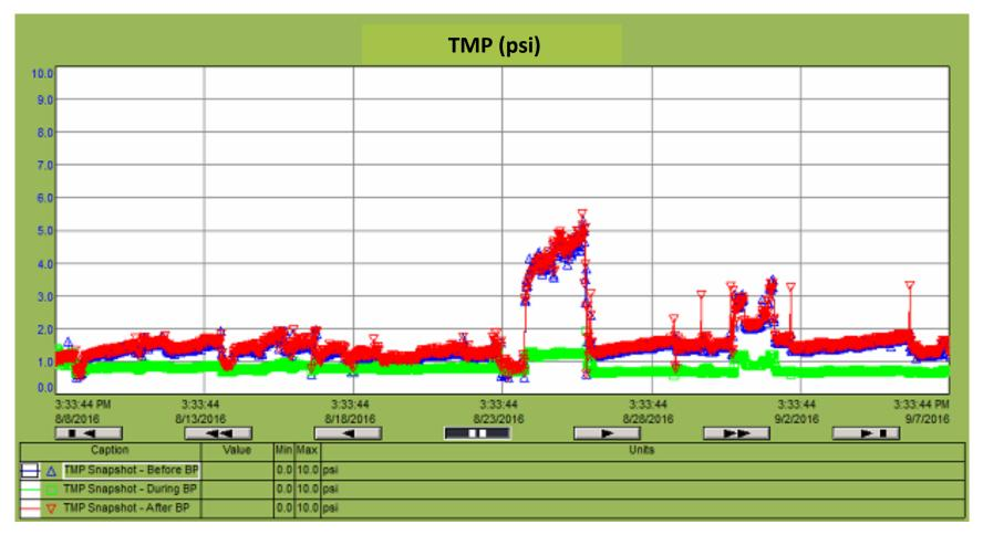
TMP of the 2 day peak test at 16.7 GFD – TMP returns to pre peak level immediately
